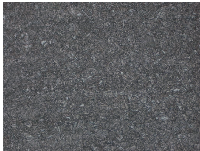
Photo Tempered Macrostructure of TP155V (x500)
